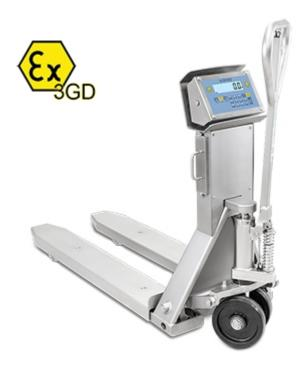
AISI 304 stainless steel pallet truck scale for use in ATEX hazardous areas 2 & 22, with Ex II 3G IIC T6 Gc X and Ex II 3D IIIC T115C° Dc X protection. Also available in approved version for legalfor-trade use.
