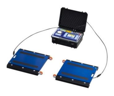
It weighs the vehicle axles and calculates the total weight. Consisting of two WWS series portable pads and the touch screen weighing terminal with integrated printer. Wired version.
