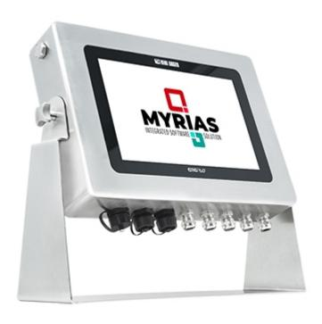
New industrial touch screen PC with an AISI 304 stainless steel case and IP67 protection degree, specifically for harsh industrial environments. It allows the loading of any weighing programme developed on Windows 10, for the creation of advanced weighing systems. High-performance Intel processor and up to 4 scale inputs.
