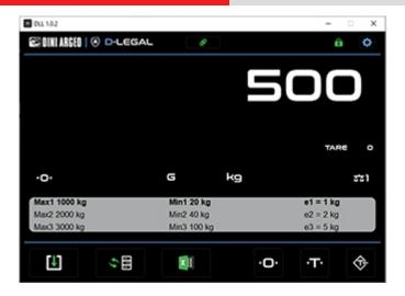
D-LEGAL software can be used to turn a PC into an approved digital weight indicator in compliance with NAWI.
