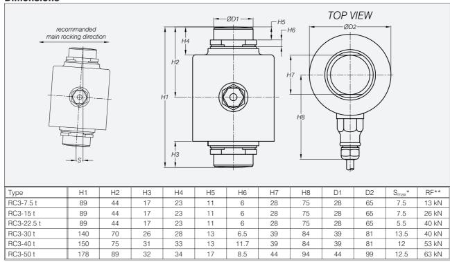
\*  $S_{max}$  = maximum lateral displacement of load introduction. Recommended gap 2...3 mm for 7.5...22.5 t, 3...5 mm for 30...50 t. \*\* RF = restoring force at  $S_{max}$  and  $E_{max}$ .
